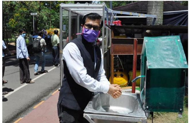
The single infrared sensor attached to the dispensing unit gets automatically activated when an object comes close to the unit.
