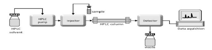
High Performance Liquid Chromotagraphy (HPLC) is an analytical technique used for the separation of compounds soluble in a particular solvent.
